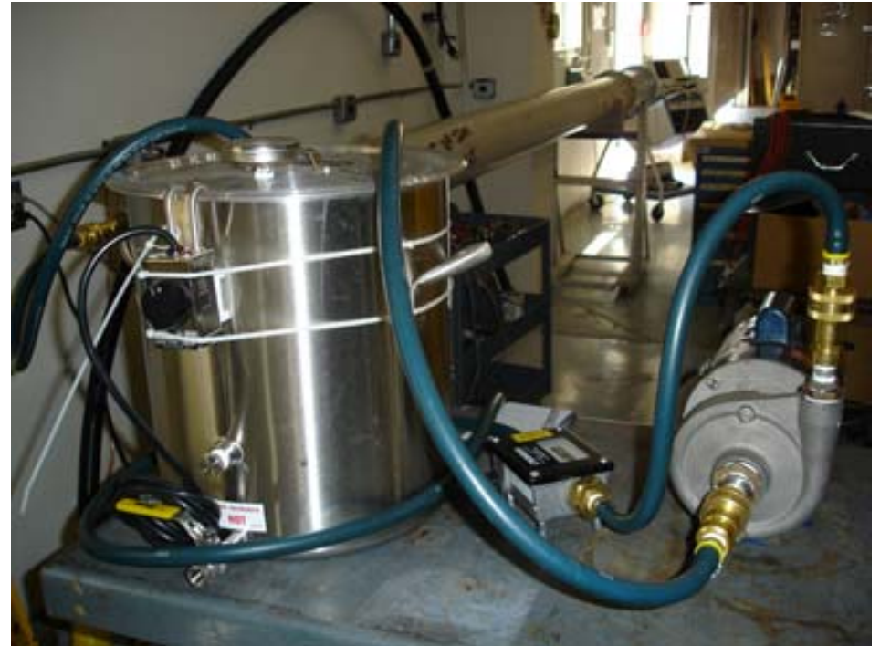
Holding tank with heater element, flow meter and pump
