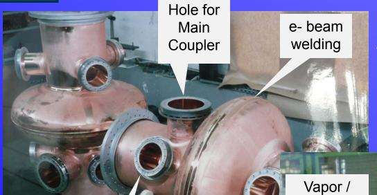
Copper 400 MHz single cell cavity
