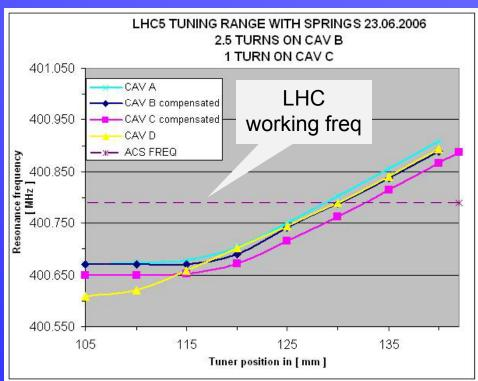
Corrected by adjustable tuning springs compensation
