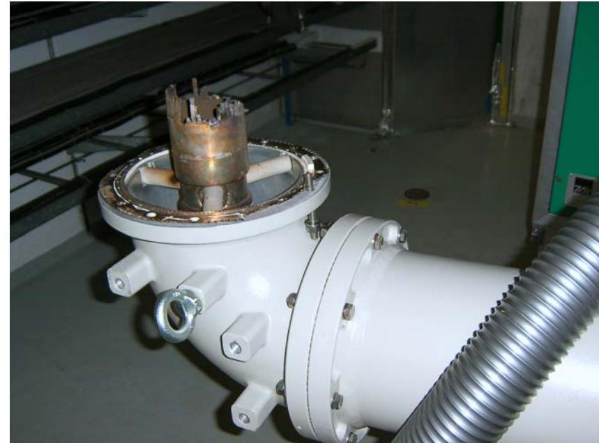
Burned finger contacts of spherical joint
