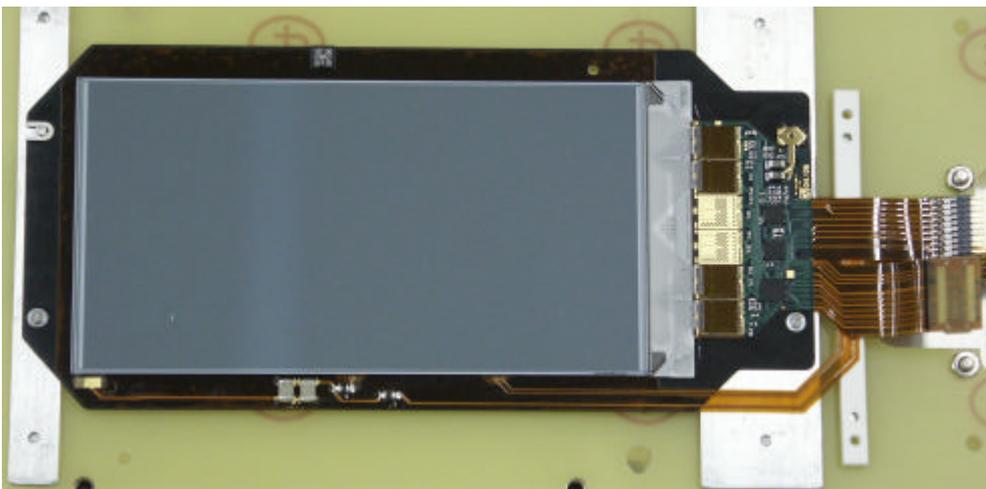
**Fig. 2** A single sided TIB Silicon strip module mounted on its test and transport carrier.
