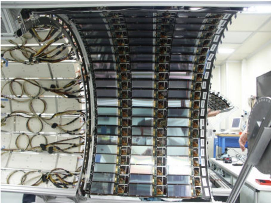
**Fig. 7** TIB layer 4, inner part, completely assembled with modules.
