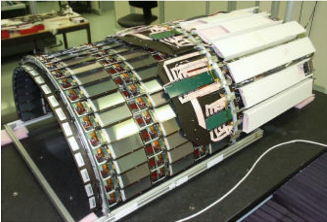
**Fig. 8** TIB layer 3 with modules and control electronics mounted on carbon fibre supports on the external part of the shell.
