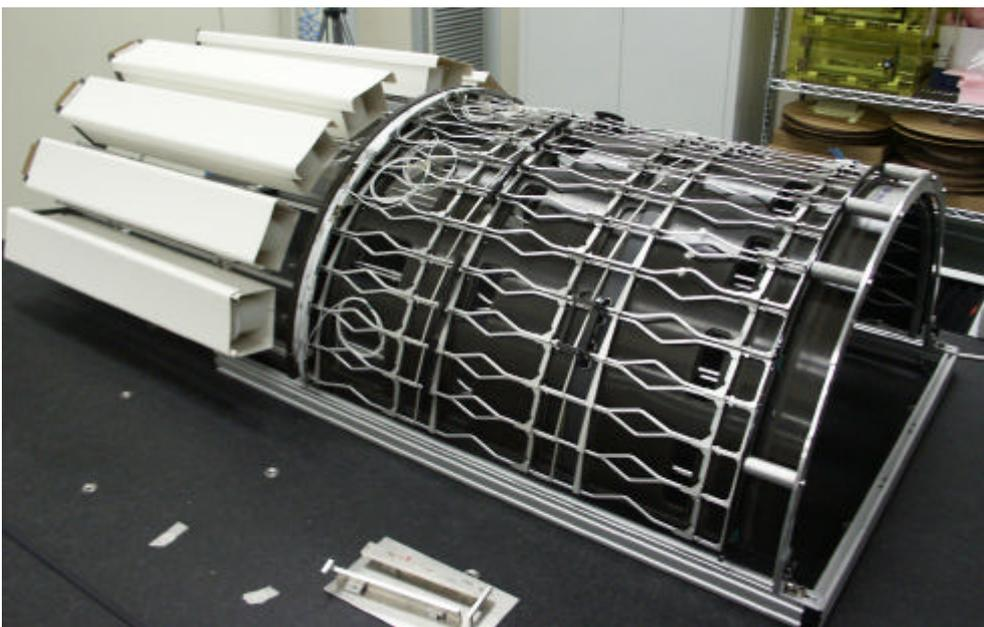
**Fig. 5** TIB layer 2 carbon fibre mechanical structure with cooling pipes and temporary optical fibre holders (left).
