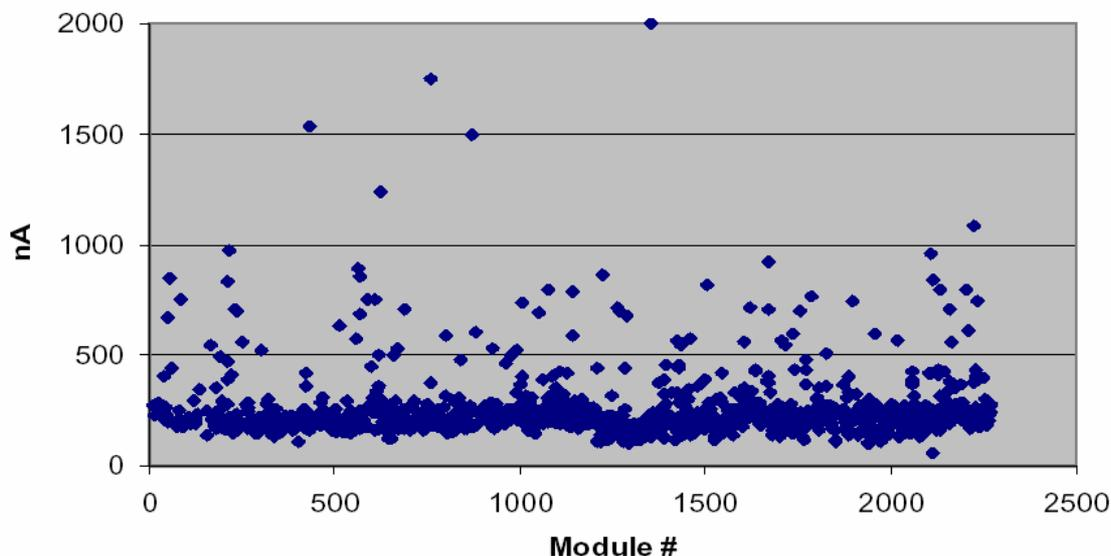
**Fig. 3** Reverse bias current, measured at 400V, for TIB modules.
