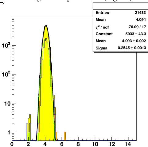
**Fig. 10** Cumulative strip noise distribution (ADC counts) of one fourth of TIB Layer 4 performed during a burn-in run using cooling fluid at -25°C. The absolute value of the noise is not normalized to the scale of neither Fig. 4 nor Fig. 9.
