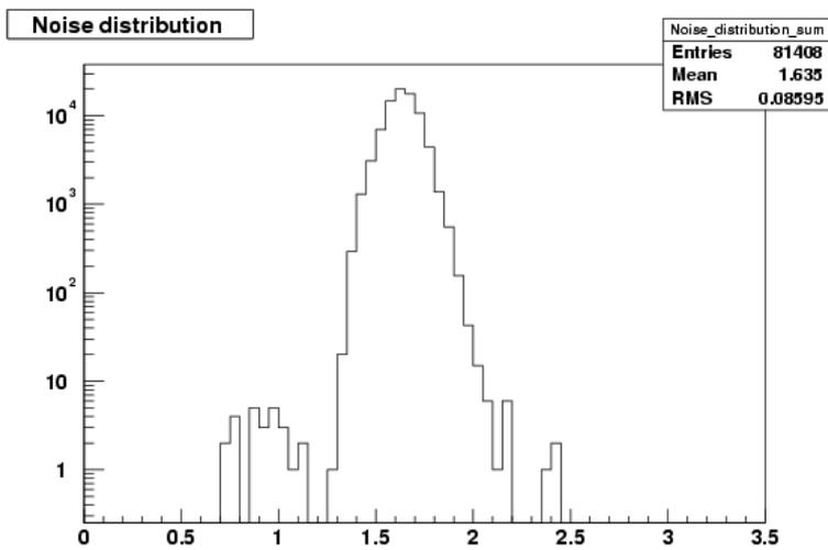
**Fig. 9** TIB layer 4 cumulative strip noise distribution (ADC counts).
