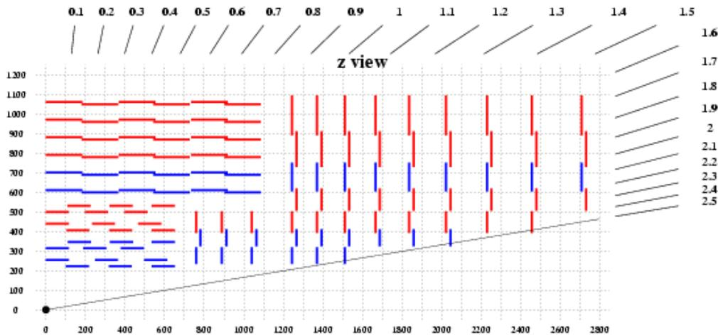
**Fig. 1** Sketch of the tracker layout (1/4 of the longitudinal view); red lines represent single sided modules while blue lines double sided ones. Dimensions are in mm, pseudorapidity coverage is also shown.
