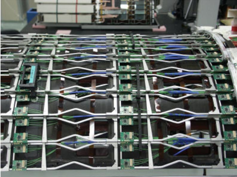
**Fig. 6** Analog optohybrids mounted on the mechanical structure.
