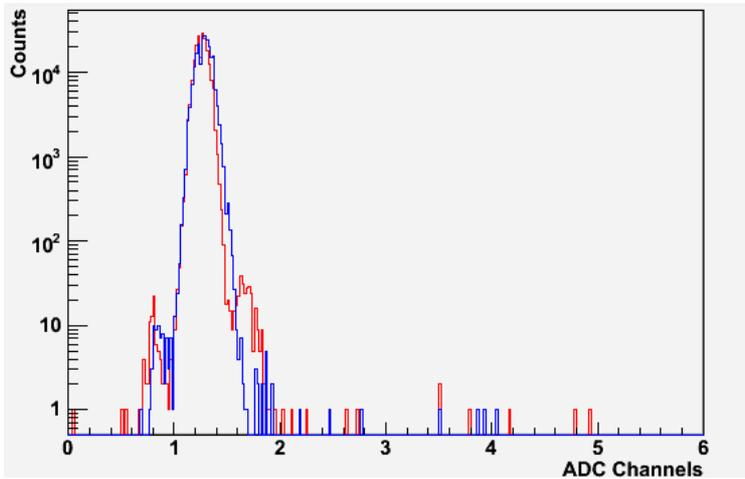
**Fig. 4** Cumulative noise distribution for TIB modules measured at  $-20^{\circ}\text{C}$  during long term test (blue: four chip modules, red: six chips modules).
