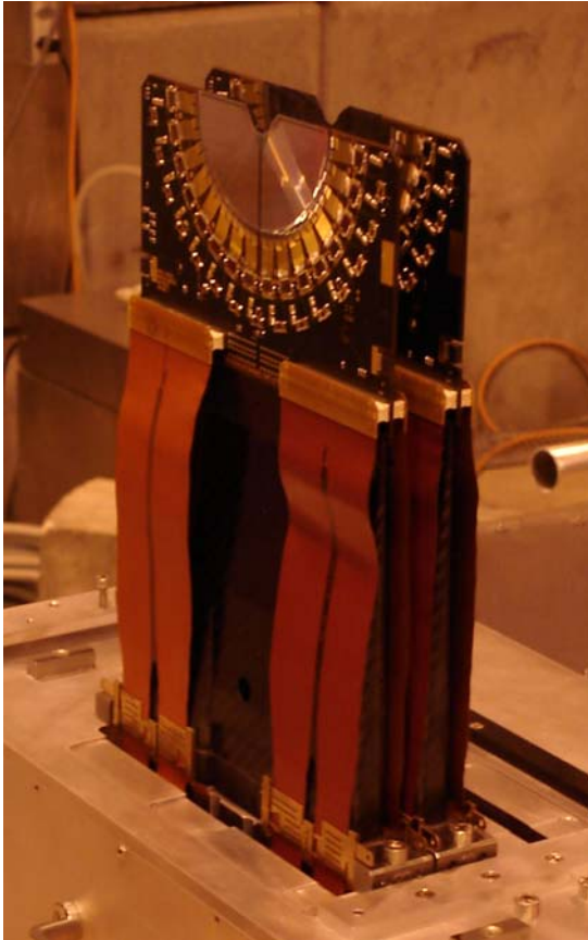
Figure 2. Picture of two complete silicon modules. Each module consists of an R and a \Phi measuring sensor which are read out by 16 Beetle chips.
