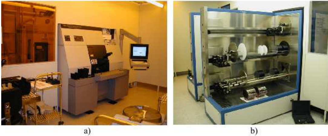
Fig. 2. Photographs of processing equipment at the LBNL MicroSystems Laboratory. a) Photograph of the projection aligner used to print patterns on 150 mm diameter wafers. b) Photograph of high-temperature furnaces used to oxidize silicon, deposit thin films, and anneal 150 mm diameter silicon wafers.
