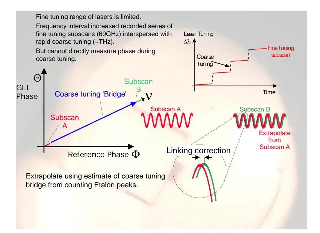
Michelson fringes will be present during scan – temperature drift Use two lasers scanning in opposite directions to cancel interferometer drift errors.
