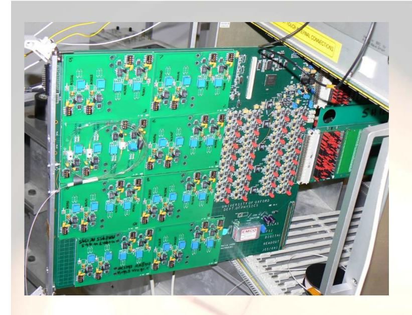
APDs, Amplifiers, 16bit ADC, 1ms time slicing, 256Mbyte store VME read-out, 64 fibres in per board – 8 x 8 way ribbon
