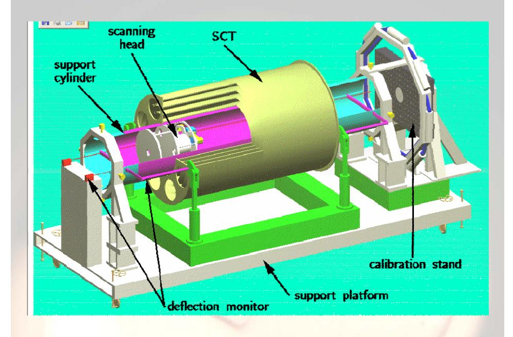
Self-calibrating using fixed strip separation to extract x-ray system parameters.
