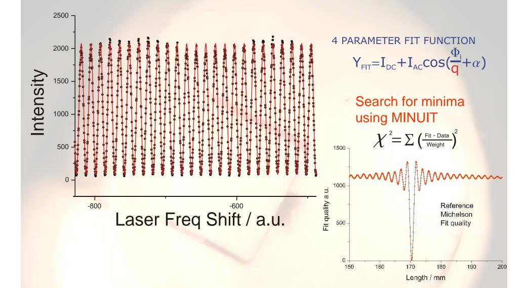
Laser frequency tuning is not linear with time so frequency is monitored during fine tuning using phase stepping in the reference interferometer:
