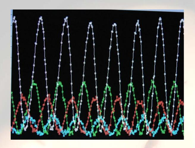
Dual laser ~pW interferences fringes from two interferometers were read out simultaneously by one APD as the optical frequency, v, was scanned (in this plot  $\Delta v$  ~ 8GHz).
