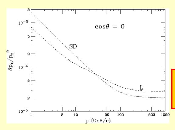
Error in radius of curvature  $\rho$  is proportional to error in  $1/p_{\perp}$ , or  $\delta p_{\perp}/p_{\perp}^2$ .
