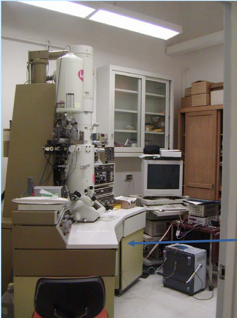
Modified GATAN bright field STEM detector housing at the bottom of the JEOL 200CX TEM
