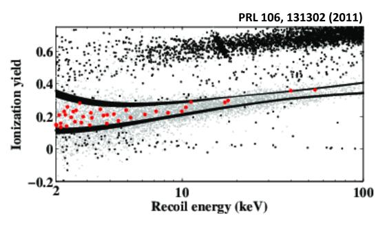
Extending the analysis of traditional WIMP search data to the trigger threshold shows that discrimination is reduced, but not eliminated at nuclear recoil energies as low as 2 keV. This figure is from CDMS-II data and the limiting background was from events where the charge signal was consistent with noise. Preliminary results show that the iZIPs have significantly reduced the quantity of events with no charge signal while retaining 2 keVr thresholds.
