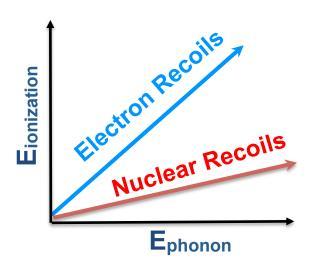
CDMS measures both the heat deposition and the ionization from particle scattering. This allows event-by-event identification the interaction as a nuclear or electron recoil down to energies below 10 keVr.
