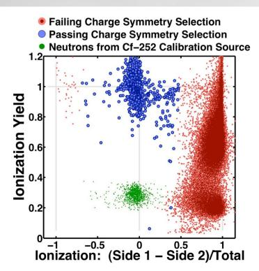
The charge is measured on both sides of the detector. With the complex electric field, the side-asymmetry in the charge collection has excellent identification of surface events. The phonon asymmetry shows similar identification of surface events.
