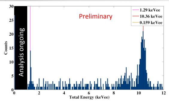
This spectrum shows the low-energy performance of SuperCDMS detectors with increased voltage. The applied bias was 69V corresponding to an order of magnitude gain in the signal. The energy resolution for the 1.29 keV gallium L-shell line is ~24 eV, the Fano limited resolution is ~20 eV. The increase at 9 keV is due to cosmic ray activation of <sup>65</sup>Zn. Note that the efficiency of the cuts used to produce this preliminary spectrum has not been applied.
