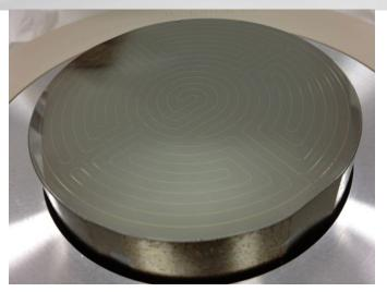
Procurement and performance testing of 100 mm x 33 mm germanium detectors is ongoing. First 100 mm iZIP has been fabricated. The proposed SuperCDMS-SNOLAB project involves fabricating and deploying 144 of these detectors.
