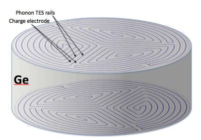
SuperCDMS iZIP detectors have phonon and ionization instrumentation on both faces allowing superior z-sensitivity.
