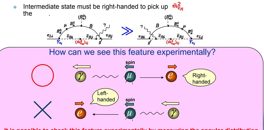
It is possible to check this feature experimentally by measuring the angular distribution of final state lepton.
