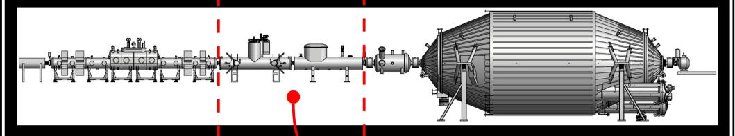
Source Section: gaseous tritium injected and removed under a high magnetic field which guides electrons
