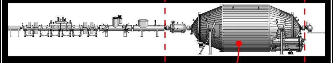
Source Section: gaseous tritium injected and removed under a high magnetic field which guides electrons
