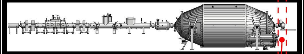
Source Section: gaseous tritium injected and removed under a high magnetic field which guides electrons
