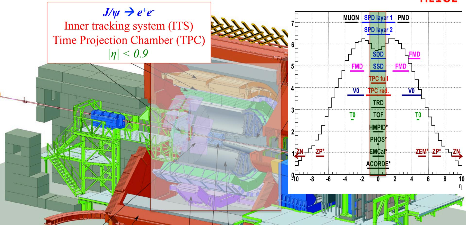
**Central rapidity:** TOF trigger requiring a hit multiplicity to be between 2 and 6, vetoing signals from both VZERO detectors, and with at least 2 hits in SPD. In addition, at least one of the triggered tracks by TOF has the angular correlation  $150^\circ < \Delta\phi < 180^\circ$
