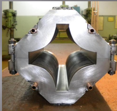
yoke of quadrupole lens after final treatment
