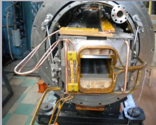
Dipole magnet in cryostat
