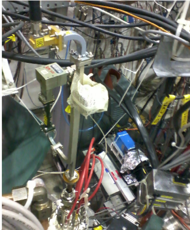
Waveguide for \mu -wave injection (UBC, SFU)
