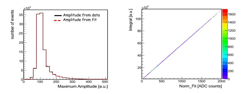
The signal shape function estimates the amplitude more accurately Good correlation between the integral and amplitude
