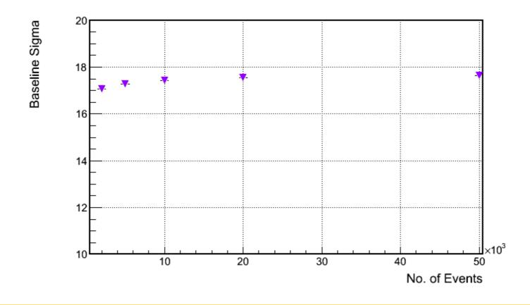
$\sigma_{Pedestal}$  is stable with respect to the number of events To save processing time - used 1000 events to estimate the pedestal width
