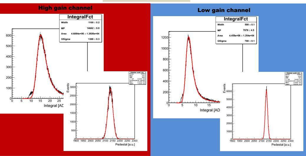
Example of SNR calculation – high gain channel: MPV<sub>Integral</sub> = 1.4662 ADC<sub>counts</sub>\*ns = 293.243 ADC<sub>counts</sub>\*sample <sub>\sigma<sub>Pedestal</sub></sub> = 17.05
