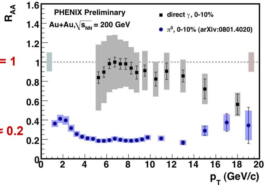
$$R_{AA} = \frac{dN / dp_T|_{Au+Au}}{N_{bin} dN / dp_T|_{p+p}}$$
