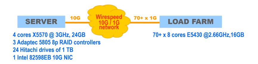
This setup reperesents well an elementary fraction of a typical large hardware installation and has basically no bottlenecks:
