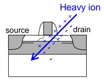
SEE = Functional anomaly or destructive effect in an electronic component, due to a single particle crossing the device.
