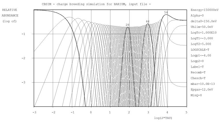
Heating rate of Ba<sup>+56</sup> in the trap 3.9 keV/s, breeding time ~ 500 ms.
