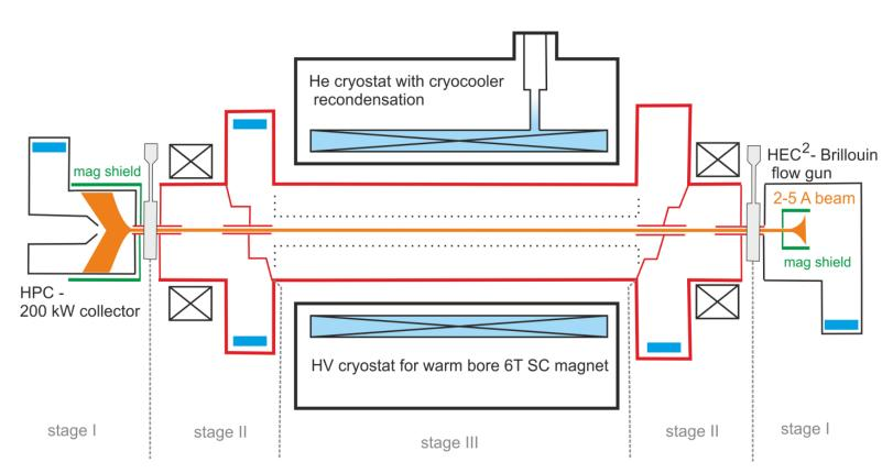
3 stages, separable, high differential, distributed pumping system with redundance
