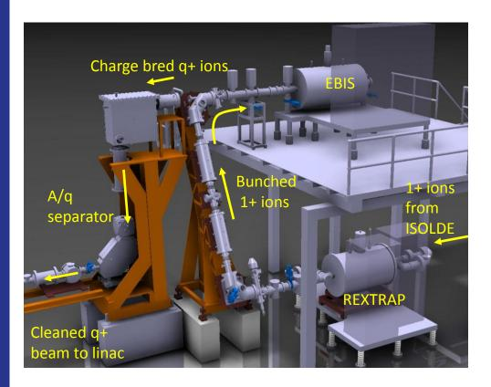
1.For a few Hz injection of high intensity beams: shoot directly to EBIS in cw due to low REXTRAP capacity of 10<sup>7-8</sup> ions.
