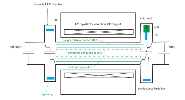
Assuming 40K shield D=100 mm, vac tube D=150 mm, length 2 m From mech. polished Steel to mech. polished Alu/Cu/Ag on Cu Radiative heat load 18/12/4 W at 40 K @ 35-40 W available on CH If NEGs have high ε combining will be impossible.
