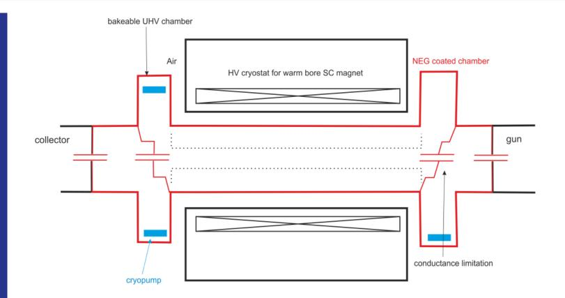
Assuming D=150 mm tube of 2 meters,  $R(H_2, NEG=Ti-V-Zr)=0.3 I/cm^2$ The total pumping rate of the trapping region = 2800 I/sec
