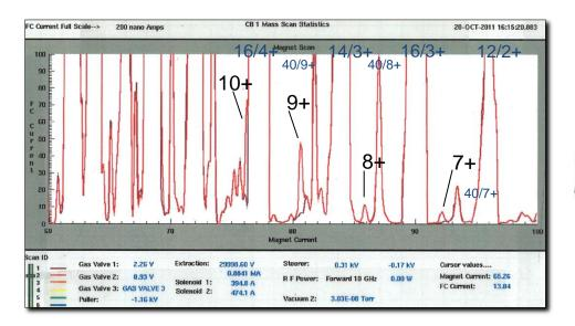
Mass scan of background plasma constituents and charge bred <sup>39</sup>K beam showing peaks for 7+, 8+, 9+, and 10+ (courtesy of Rick Vondrasek). Post-accelerated <sup>141</sup>Cs RI beam
