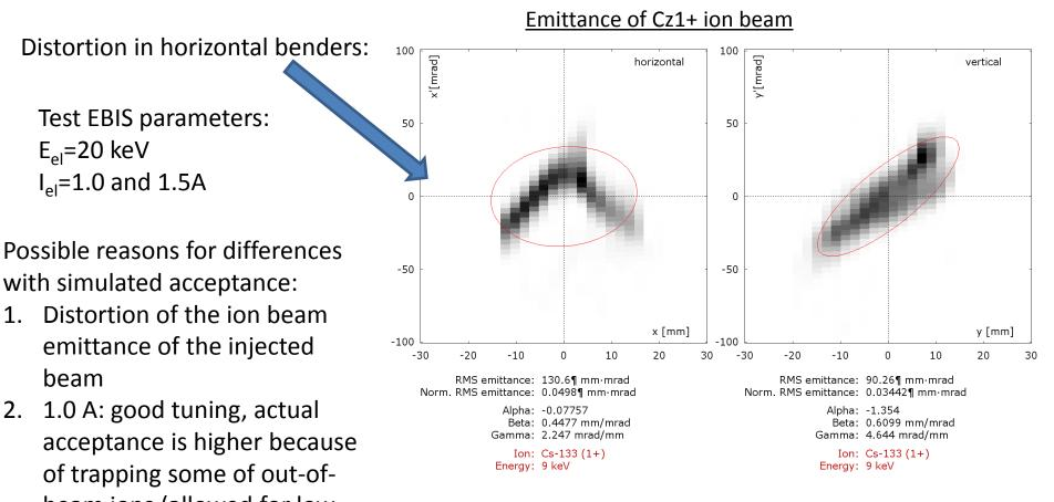
beam ions (allowed for low neutralization)3. 1.5A: not sufficient tuning
