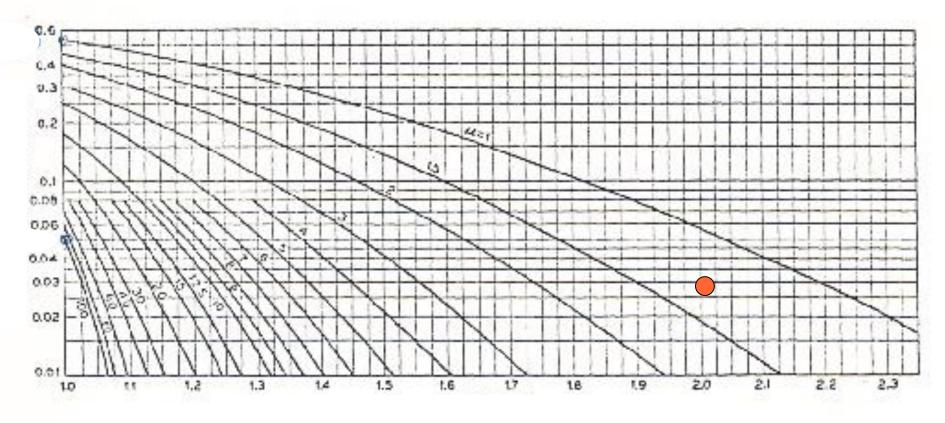
The parameter  $\mu$  is the potential depression over the beam temperature, which is about 1.33 for the 5 A, 20 kA/cm<sup>2</sup> beam under consideration. 3% of the beam is outside of twice the beam radius which is about 0.1 mm.
