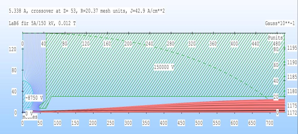
The beam is well focused and well immersed, which is the result of relativistic aid in focusing.
