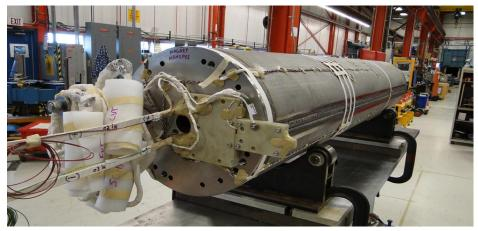
The magnet reached 10.4 T or 78% of SSL at 1.9 K
