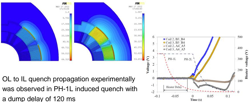
Quench propagates from OL to IL in ~ 80 ms at 62 % of SSL
