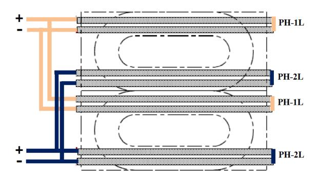
PH-1L and PH-2L heaters from both coils are connected in parallel to a separate Heater Firing Unit (HFU)
