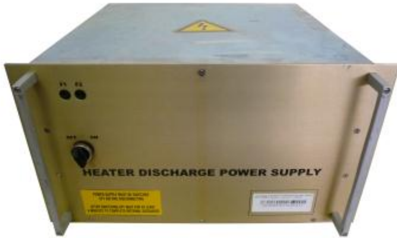
6076 quench heater power supplies.
