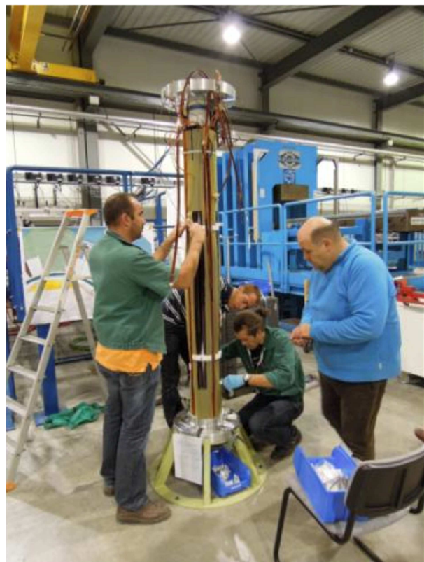
Fig. 1: Vertical assembly of the coils around the collapsible mandrel, and open ground insulation around the coils.
