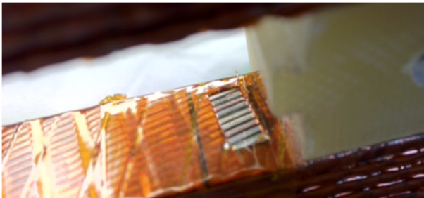
Fig. 4: A view of the quench heaters with their cooling slots mounted between layers. We also see the spot heater and adjacent voltage taps.
