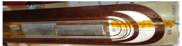
Fig. 8: Inductive loop formed by the voltage taps coming from the interlayer joint in MQXC1.
