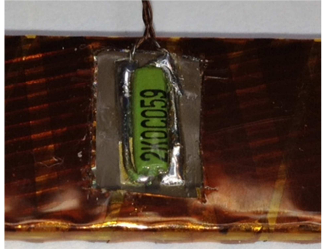
Fig. 7: CCS temperature sensor mounted directly on cable. The sensor has a 0.025mm thick kapton film insulating it from the coil yet maintaining a rapid thermal response to temperature change during measurement.
