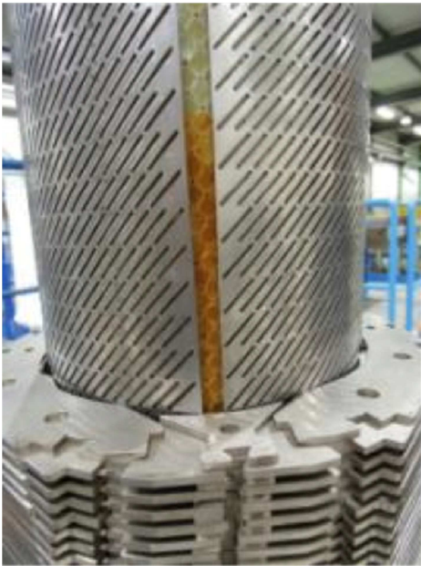
Fig. 2: Assembly of the collared coil: view of collars before compression, and collaring shoes with openings.
