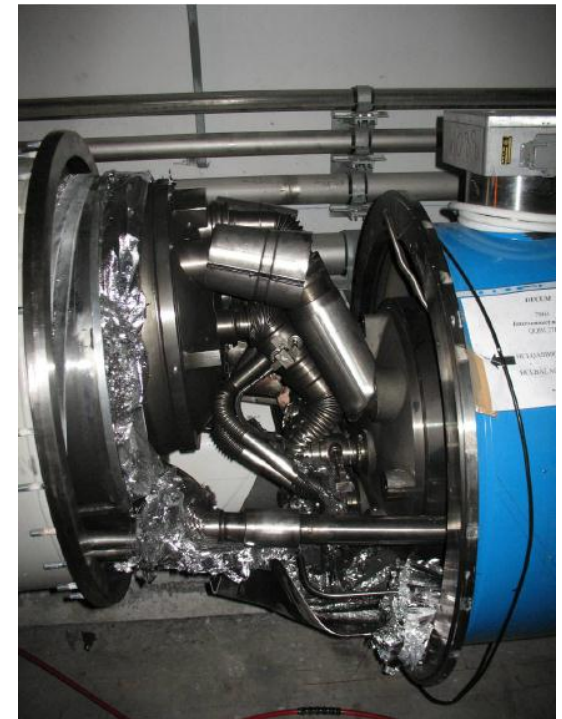
This is the result of a chain of events triggered by a quench in an LHC bus-bar
