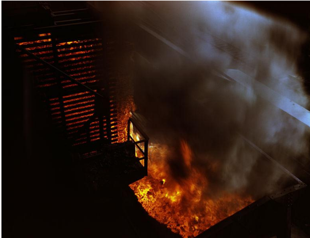
Coke being pushed into a quenching car
