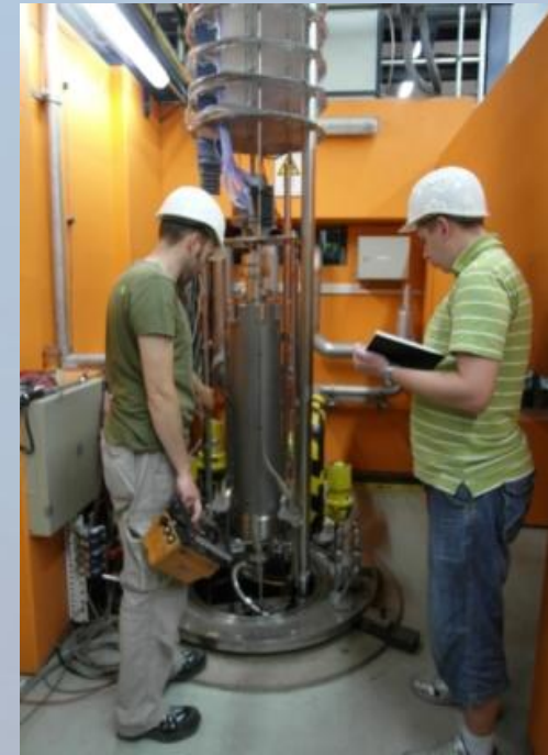
Installation of RF cavities in the vertical cryostat
