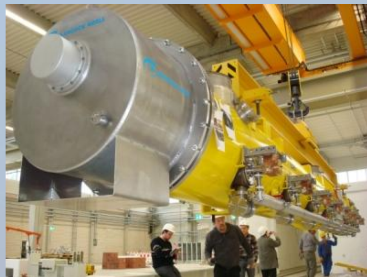
Transportation of the prototype cryomodule to the test stand
