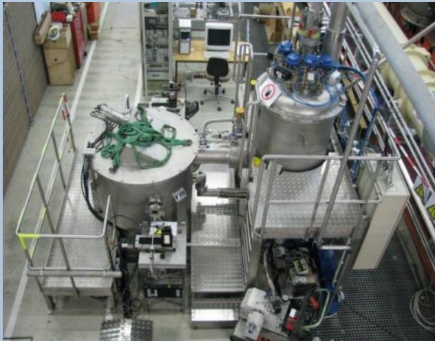
Setup for tests of magnets (left), quadrupole inside the cryostat vessel (right)
