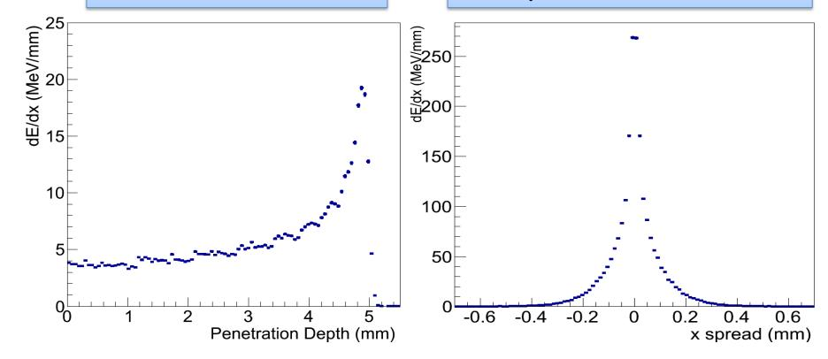
30MeV protons can penetrate 5mm of silicon and have a very small transverse position spread
