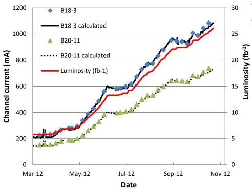
Current is monitored at the power supplies. Hamburg model is used to calculate the evolution with the luminosity, time and temperature.
