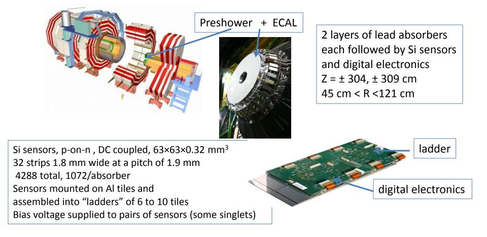
Ladders mounted on the absorber, cooled with C<sub>6</sub>F<sub>14</sub> Temperature measured by the detector control units on the hybrids 1072 measurements per absorber plane
