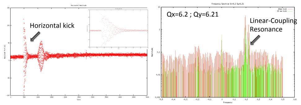
An automatic application is being developed by PS-operators to be able to measure for all reachable tunes.
