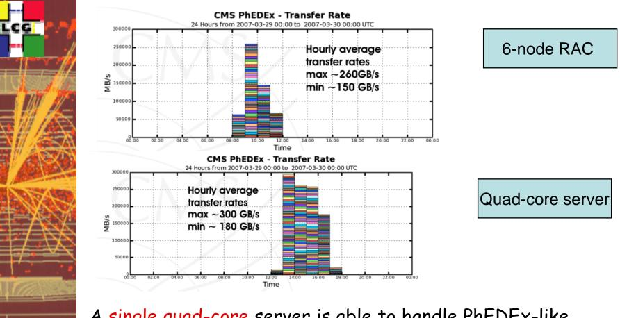
A single quad-core server is able to handle PhEDEx-like workload (a transaction oriented application) even more efficiently then a 6-node RAC
