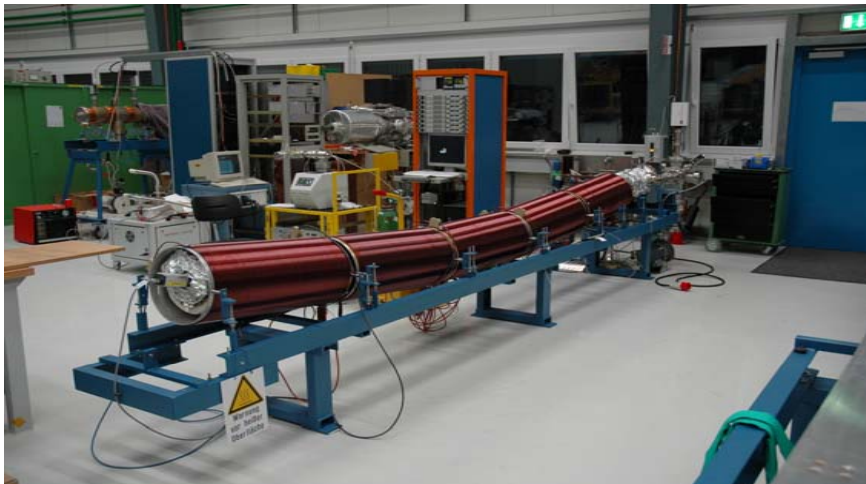
Collimators and NEG coating suppression of desorption and strong pumping
