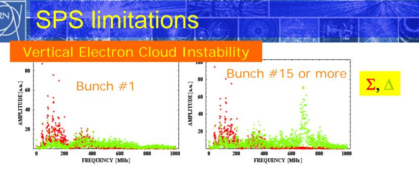
TMCI-like instability (~700 MHz) affecting trailing bunches at injection above the threshold for electron multipacting (typically 0.8-0.9 × 10<sup>11</sup> p/bunch after scrubbing). Cure: Large  $\xi_V \rightarrow$  Lifetime
