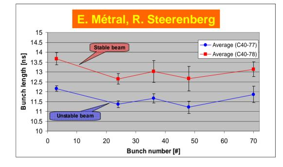
Electron-cloud instability observed for bunches shorter than 12 ns in 2006 for the nominal bunch intensity.
