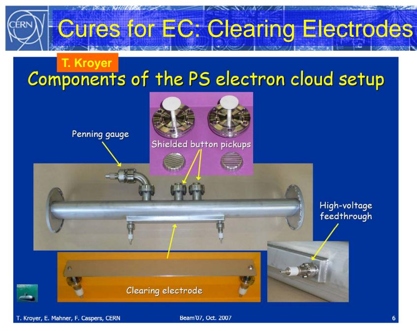
**Cures for EC: Clearing Electrodes**
