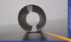
testing the deposition of enamel strips inside a beam pipe...
