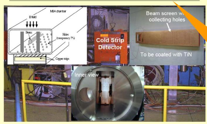
Tests with beam in the machine environment is necessary to qualify the coating as EC killer. These studies will be beneficial also for the PS2 upgrade!
