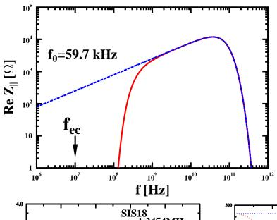
Real part of the longitudinal resistive wall impedance on the excitation frequency for  $f_{\rm ec} = 10$  MHz ( $n_{\rm ec} = 10^{12}~{\rm m}^{-3}$ , KEKB LER). Blue line: impedance without electron cloud
