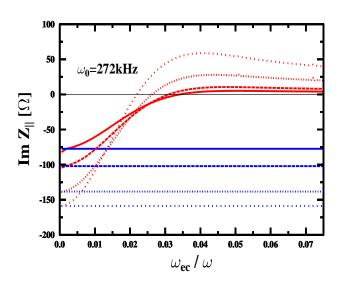
Imaginary part of the longitudinal resistive wall impedance (SIS18 left, high energy ring right)
