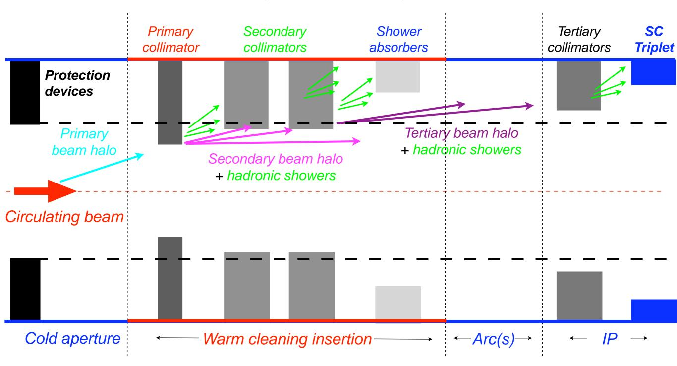
All cleaning + protection devices must be included in simulations!
