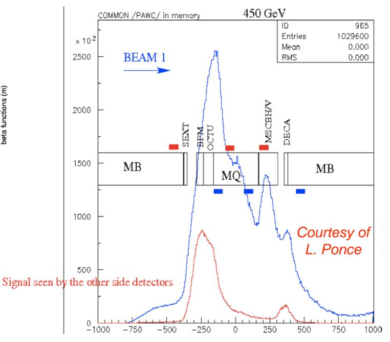
Final layout: 6 monitors per quadrupole + dedicated monitor (dispersion suppressor downstream of IR7)
