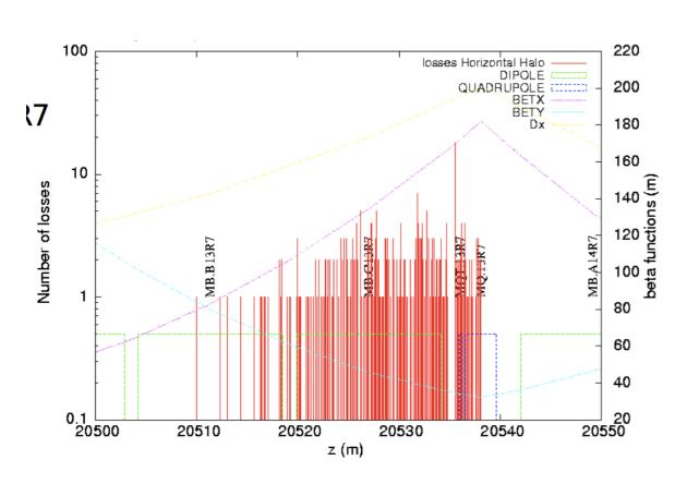
Detailed loss maps around the ring used to determine the location of the beam loss monitors (BLM s)
