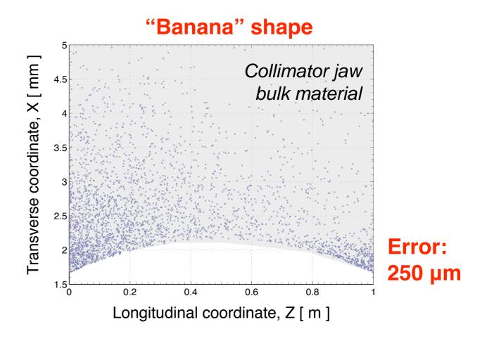
Simulations: can slice each collimator and assign any shape (polynomial fit)
