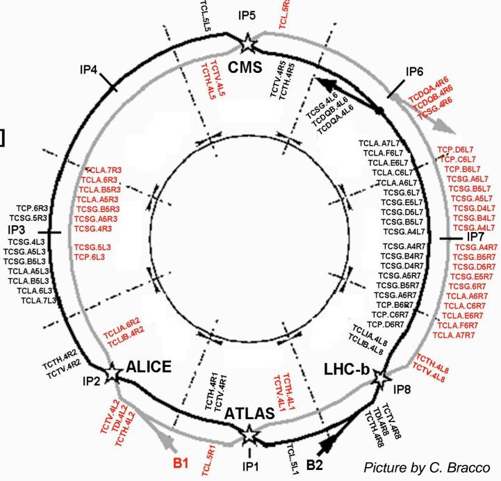
44 movable ring collimators per beam for the Phase I system!
