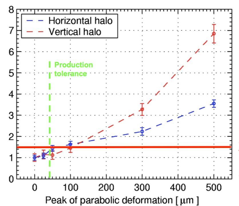
Based on these studies, the production tolerance was set to 40 µm.
