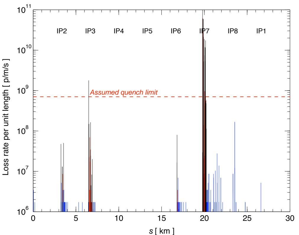
Larger losses (larger betatron amplitudes at lower energy) but also larger quench limits.
