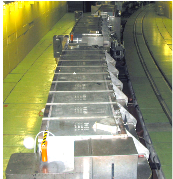
Figure 4: PS main magnet units. The ACEM BLM detectors are the orange cylinders mounted on top of the magnets.
