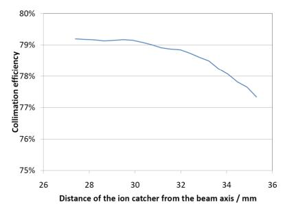
Calculated for only 10 installed collimators, two sections cannot be used because of non-moveable insertions (extraction septum and ion cooler).
