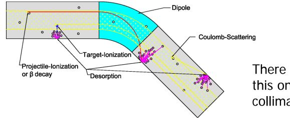
There are more loss processes, but this one can be controlled with collimators / catchers!
