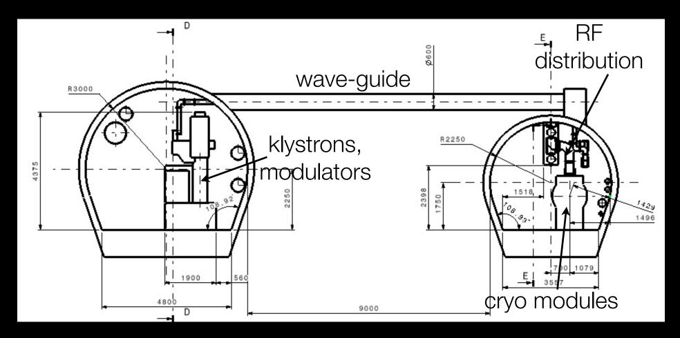
klystron tunnel (diameter: 6 m) accelerator tunnel (diameter: 4.5 m)
