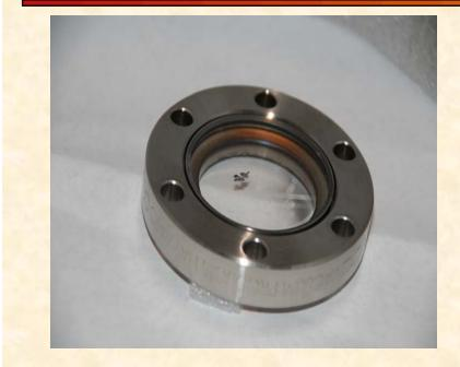
Powerful laser breaks the windows – in our experiment the laser density was reduced by factor 2 to prevent window damage. The maximal efficiency achieved when laser power increased to maximum and laser spot area increased two times
