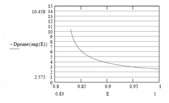
Needed dispersion derivative is a very nonlinear function of energy. 840 MeV – absolute minimum for 355 nm. In reality 950 MeV is already a problem for optics. Contrary to first experiment, We need 1 GeV to get Needed dispersion.
