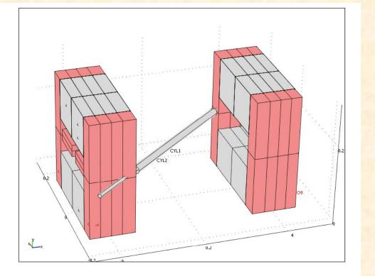
Main reason for new magnet design there is no possibility to shrink the vacuum chamber aperture because of risk to interfere with neutron production The idea is to use permanent magnets (NdFeB), combine them with laser optics, make it movable, and put whole system in vacuum chamber
