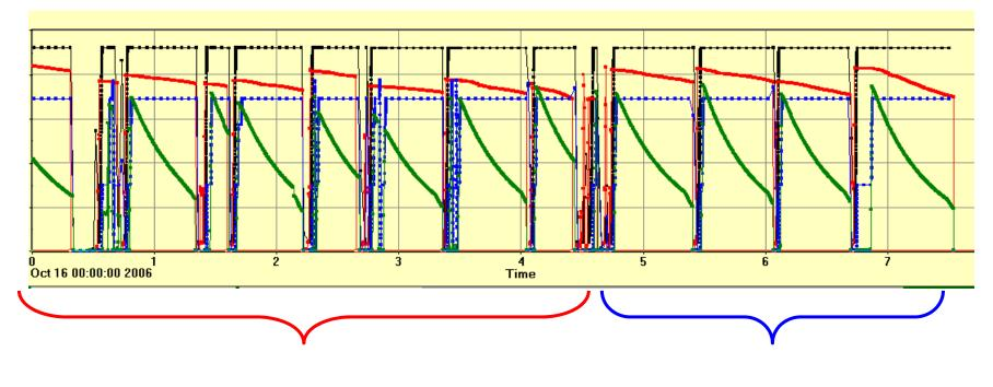
exclusively unscheduled p beam losses unexplained proton beam losses beam shower in collimation section fast losses: ms regular operation
