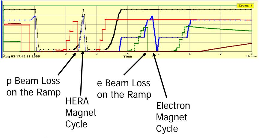
$\rightarrow$  5.5 hours from beam dump to luminosity
