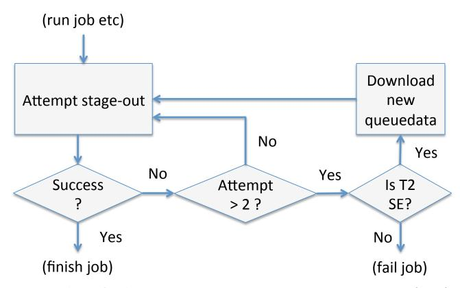
In case pilot fails to stage-out at primary SE (T2), download new queuedata from schedconfig and reattempt stage-out to secondary SE (T1 in the destination cloud).
