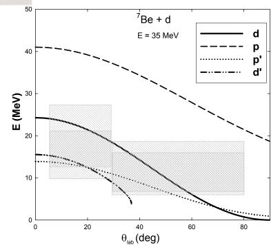
Kinematics of the 7Be(d,d), 7Be(d,p) reactions for ground state (d) (p), excitation of 20 MeV (p'), 5 MeV (d') respectively. The forward hashed (backward hashed) areas cover the detected p (d) energies and angles in CD and barrel detectors of T-REX.
