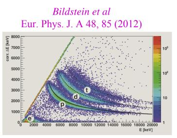
Energy resolution of T-REX would be sufficient for particle identification in this experiment
