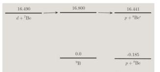
FIG. 1. Schematic illustration of the proposed <sup>7</sup>Be destruction mechanism,  $d + {}^{7}\text{Be} \rightarrow {}^{9}\text{B}^{*} \rightarrow p + {}^{8}\text{Be}^{*}$ . The energies are in MeV relative to the ground state of  ${}^{9}\text{B}$ . Subsequently,  ${}^{8}\text{Be}^{*}$  breaks up into two  $\alpha$  particles.
