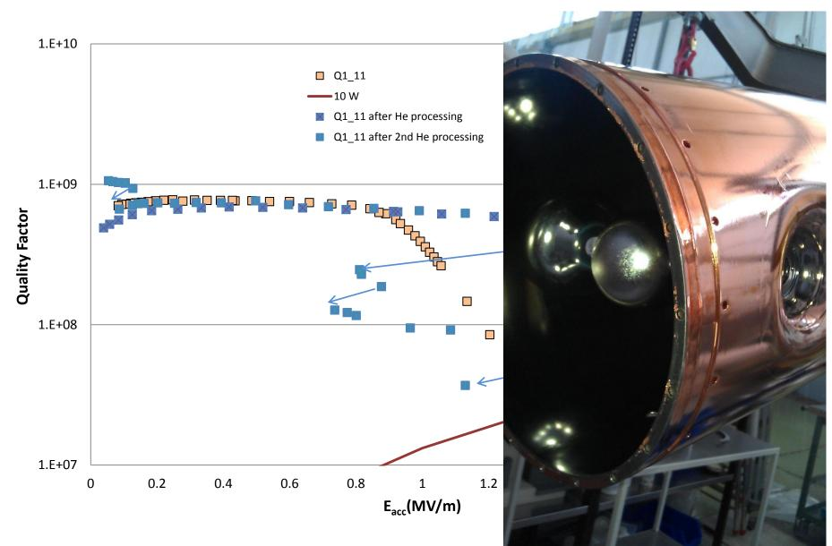
QP1 test results: before He processing, similar behaviour as Q1\_11 after He processing. Onset al lower fields. Slight gain in field at 3 K
