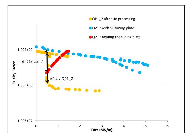
Power dissipation due to a normal conducting bottom plate (flat plate Tipgap70)@0.55MV/m: calculated value Δpcav@0.55MV/m= 0.11455W\* QP1\_2 Pcav@0.55MV/m = 0.041W before
