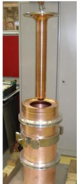
1 cavity (Q4) manufactured for sputtering tests on samples
