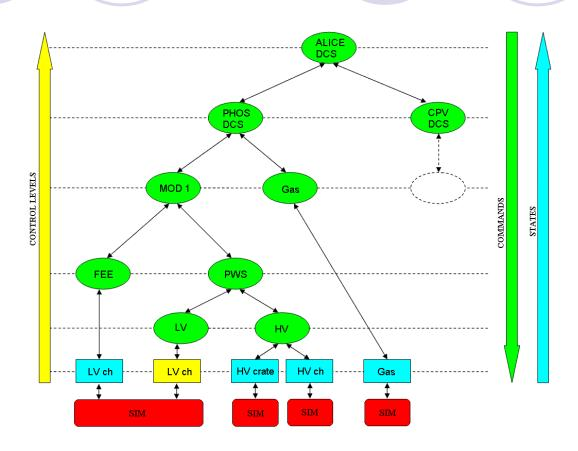
Detector control system of PHOS calorimeter is an hierarchy system which includes devices (blue color) and supervisory levels (green). Simulators (red) model the real devices' behavior and form an independent hardware abstract level.
