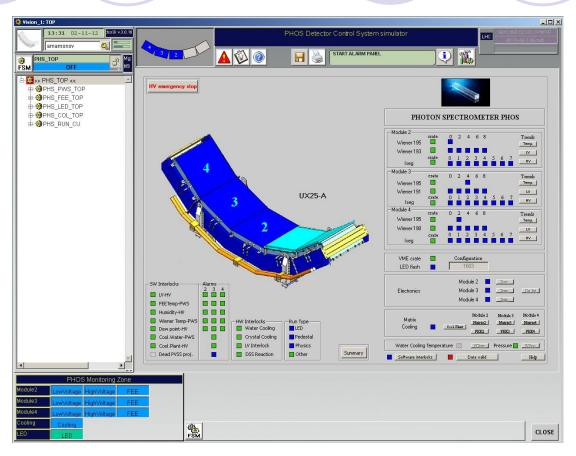
The detector control system contains: users' interfaces, a system of rights and access, diagrams, a system of control over connection with devices, an alerting message system, a software and hardware detector protection system, a detector's automatic configuration system depending on the run type.
