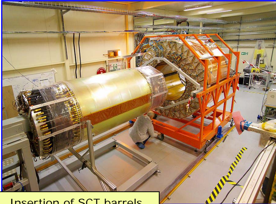
Insertion of SCT barrels within the TRT (Feb 2006)
