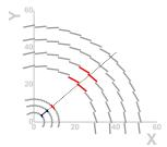
The SiTrack algorithm follows a combinatorial pattern recognition strategy, arranging the Pixel and SCT space points in "logical layers". corresponding to sets of detector layers.
