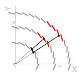
The SiTrack algorithm follows a combinatorial pattern recognition strategy, arranging the Pixel and SCT space points in "logical layers". corresponding to sets of detector layers.
