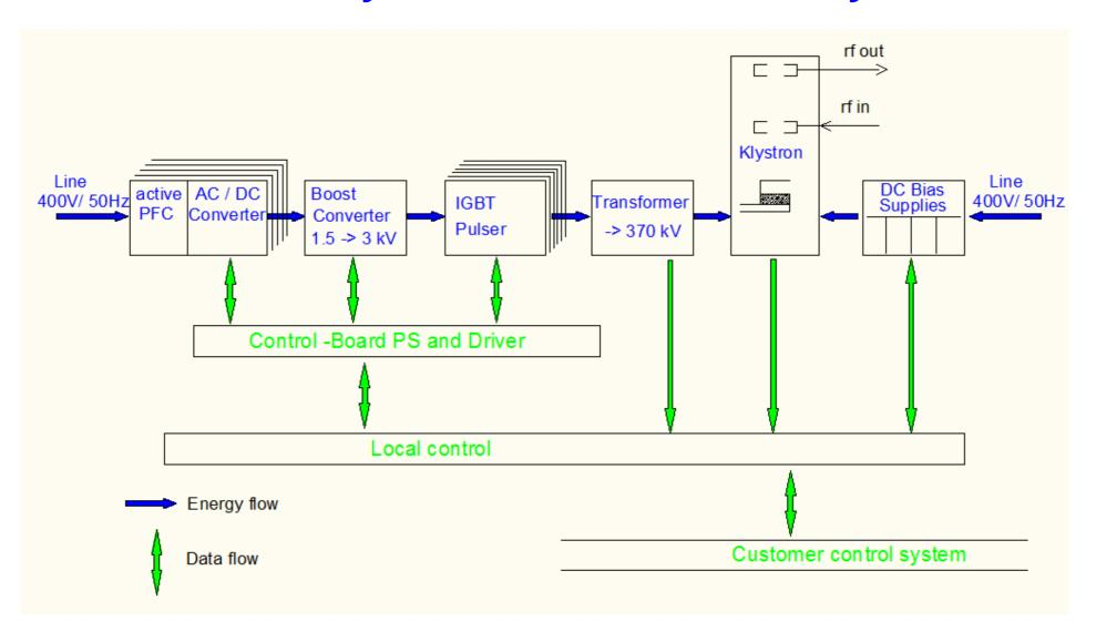
**Short-Pulse Klystron Modulator: PP-IGBT Module**
