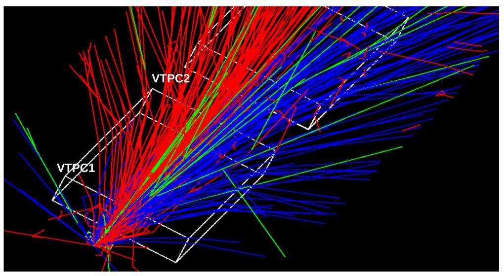
$\rightarrow$  VTPCs filled with Ar-CO2 mixture, location and dimensions as in Na61 setup.
