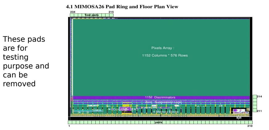
$_{\square}$  The readout speed of the whole fame in  ${\sim}100~\mu s$  (10 kHz), zero suppression circuit.
