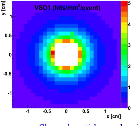
We can expect very high hit occupancy on the level of 5 hit/mm<sup>2</sup>/event in the most inner part of the vertex detector.
