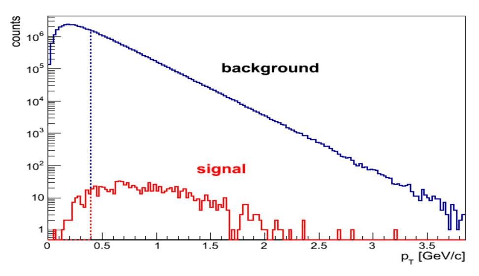
Background pT spectrum has maximum around  $\sim 0.2$ GeV/c, wheres maximum of signal distribution is at around 1 GeV/c
