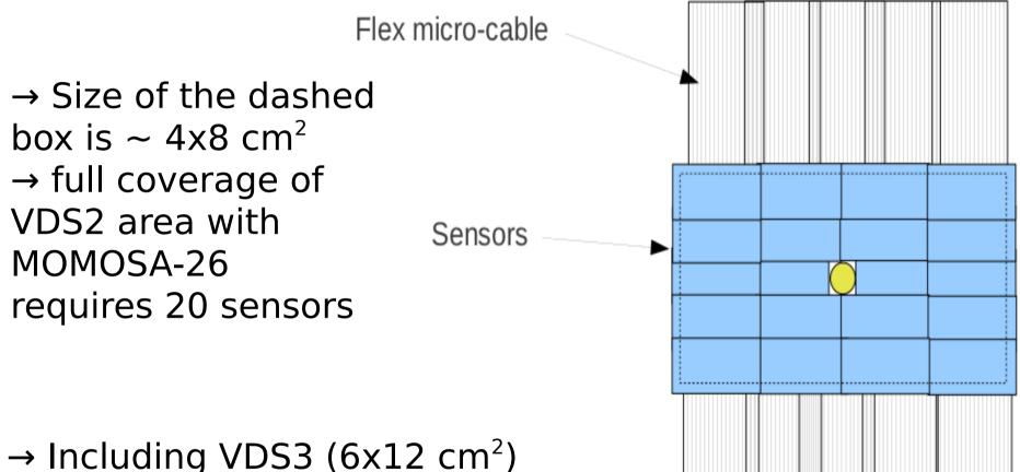
→ Including VDS3 ( $6x12 \text{ cm}^2$ ) and VDS4 ( $8x16 \text{ cm}^2$ ) we will need about 120 sensors for the whole detector.
