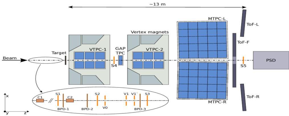
**Beam detectors and triggering**  $\rightarrow$  A set of upstream scintillator and Cherenkov counters and beam Position detectors provides timing reference, charge and position measurements
