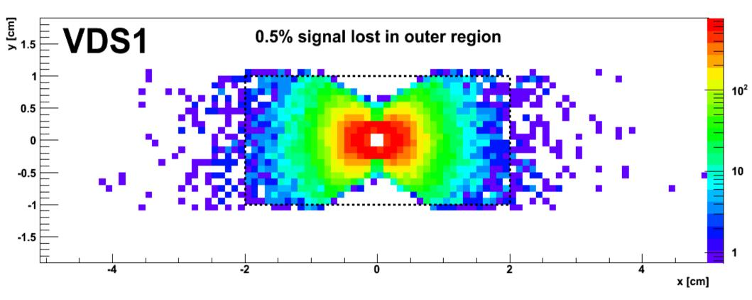
The figure shows hits (x,y) distribution generated by signal tracks is Vds1. The dashed boxes represent the cuts. We found that ~99.5% of signal tracks is localized within the box 2x4 cm<sup>2</sup> As we can see, to cover the remaining 0.5% we would need to extend the cut in the x direction for almost factor of 2.
